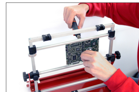
Unsoldering of components carried out with PC Assembly Jig in vertical positions.
