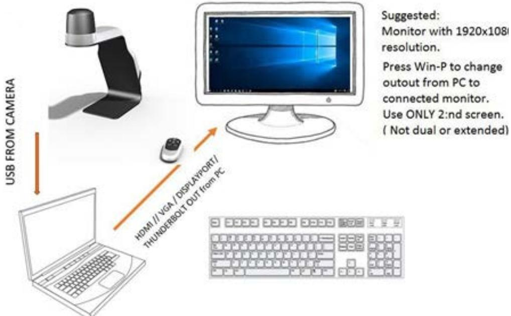
**DO NOT CONNECT THE DEVICE BOTH TO A MONITOR AND PC TOGETHER.**
