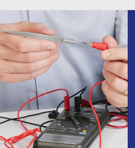
Testing tweezers have a special banana connector molded on their tails. By connecting a red cable to one tweezer and a black cable to the other, they transform into two precise measuring probes, offering the precision of a Swiss-made tool. This design allows you to grasp and measure the wire accurately with your classic LCR meter.
