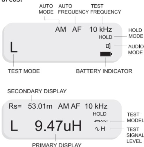
**PRIMARY DISPLAY:** The Primary Display is located in the middle of the screen and uses the largest font. It shows the dominant impedance parameter reading typically with 5 digits displayed.
