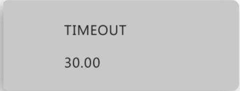
Select TIMEOUT to adjust the timeout before the unit goes to sleep mode. Move Navigation Control UP or DOWN to change the timeout value (10sec – 200sec) PRESS to exit the menu..
