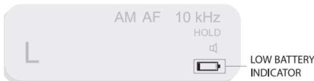
The empty battery icon on the display indicates that device's battery voltage is low and it should be recharged. The warning appears when the battery voltage drops below 3.55V, i.e. the batteries are about 90% depleted. The unit is still operational for a short time; however the batteries should be recharged as soon as possible
