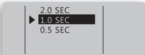
Period menu is used to set the time period between measurements. This setting does not affect measurement accuracy.
