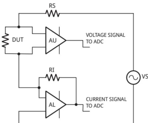
Voltage across the component is generated by the test signal source  $V_s$ . Both the amplitude and frequency of  $V_s$  can be set. The voltage is applied to the device under test (DUT) through the source resistance  $R_s$ . Current flows to the virtual ground of the current amplifier  $A_I$ , and through the current conversion resistor  $R_i$ . The output of  $A_I$  provides a signal proportional to the current,  $I \cdot R_i$ .
