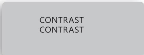
Select CONTR to adjust display contrast. Move Navigation Control UP or DOWN to change contrast. PRESS to exit menu at the adjusted contrast level.
