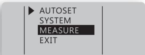
Main menu is used to access System menu, Measurement menu or to restore measurement parameters to the default state using Autoset.
