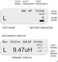
**PRIMARY DISPLAY:** The Primary Display is located in the middle of the screen and uses the largest font. It shows the dominant impedance parameter reading typically with 5 digits displayed.
