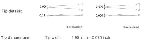
dimensions:Tip width1.90 mm - 0.075 inchTip thickness0.11 mm - 0.004 inch
