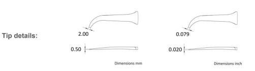
Tip dimensions:Tip width2.00 mm - 0.079 inchTip thickness0.50 mm - 0.020 inch
